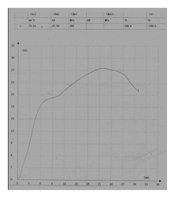
The D ring failed at 27.59 kiloNewtons which converts at 6202lbs or 2800Kg in a static pull
